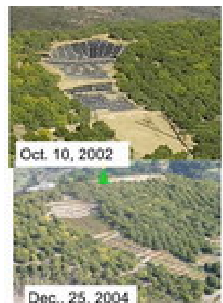
Protection of mudslide area in southern California using vetiver grass – photo by Jerry Coyle
